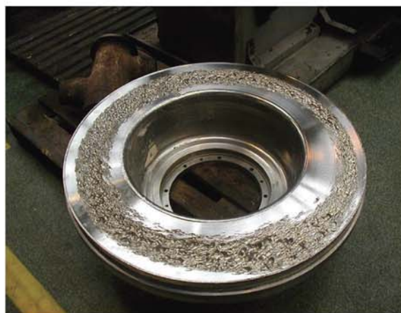
Figure 2 Abraded Throat Bushing
