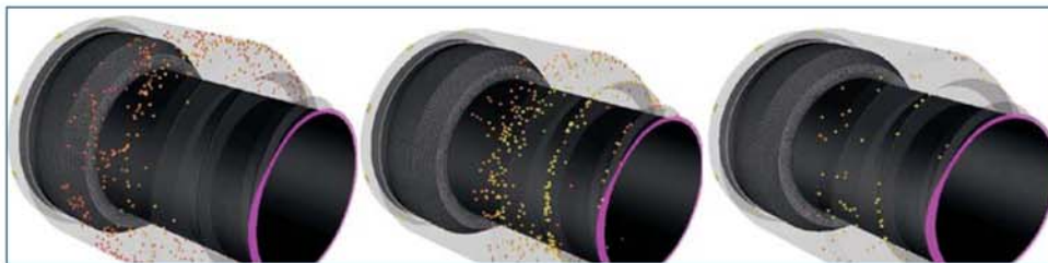
Figure 3. Time progression showing dispersion of solids by spiral grooves.
